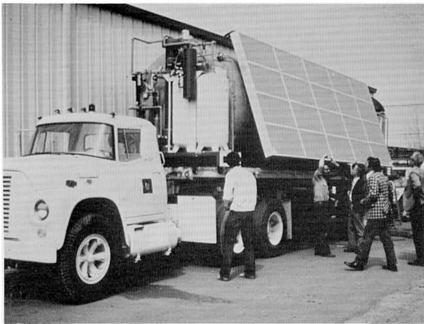
This rig converts cattle manure into clean, burnable methane gas in less than two weeks. It toured the Southwest demonstrating the energy potential of feedlot wastes. (Photo courtesy Colorado Office of Energy Conservation.)
